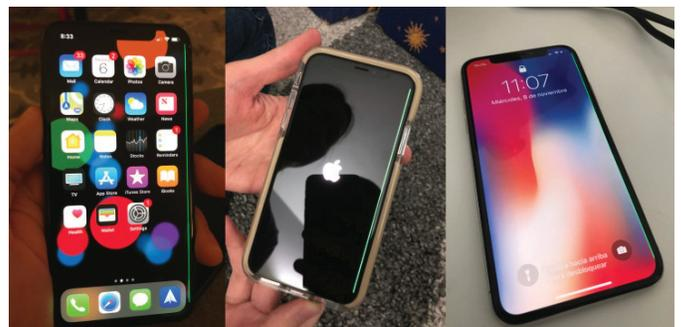
We can at least speculate on one part of that. iPhone Xs have a new diamond sub-pixel pattern in their displays, and as such all green sub-pixels appear in lines, while red and blue alternate.
